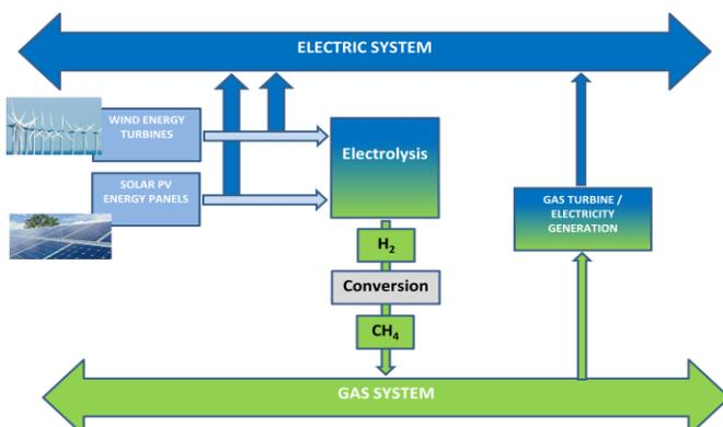
*Hydrogen is the basic element in Power-to-Gas technologies*
